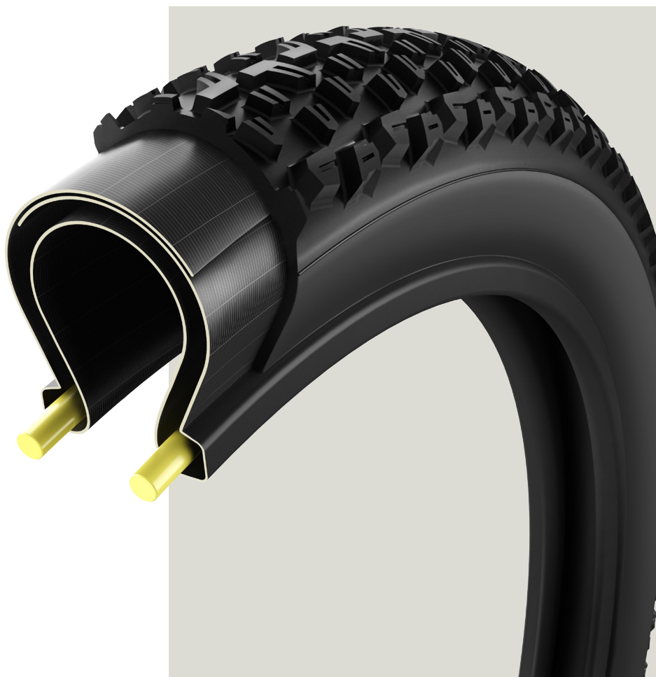
FIGURE 6. An example of tubeless construction.
